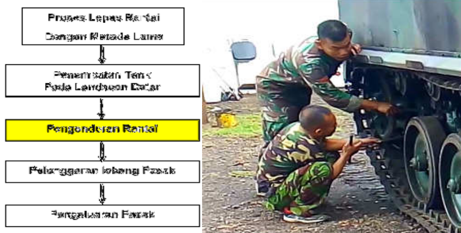
Gambar 4.3 Pengondoran Torsi Penegang Rantai
