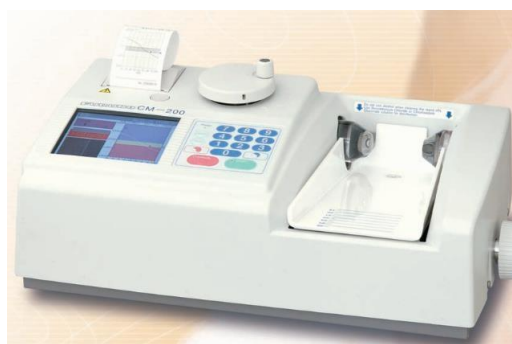
Gambar 2. 4 Instrumen QUS, CM-200 (CMDS)
