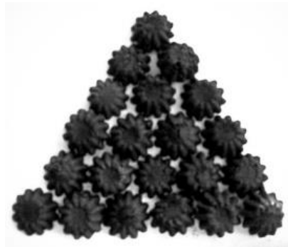
Gambar 4.7 Besi Pellet/Besi Sponge Campuran Silika Hasil Proses Microwave
